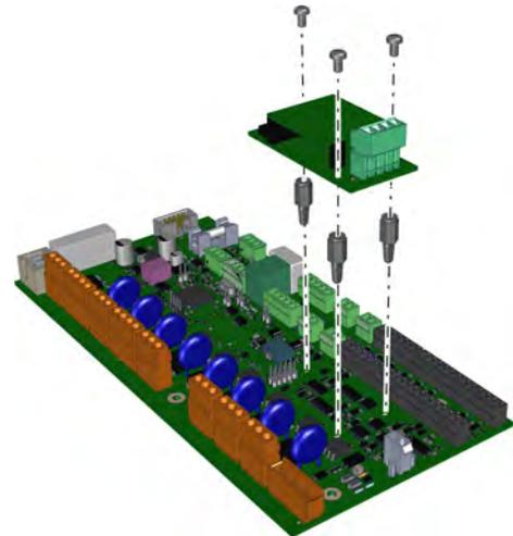
Fig. 3-5: M-bus circuit board for heat flow meter
