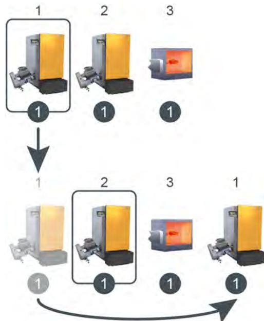
Fig. 3-2: Boiler order with burner
