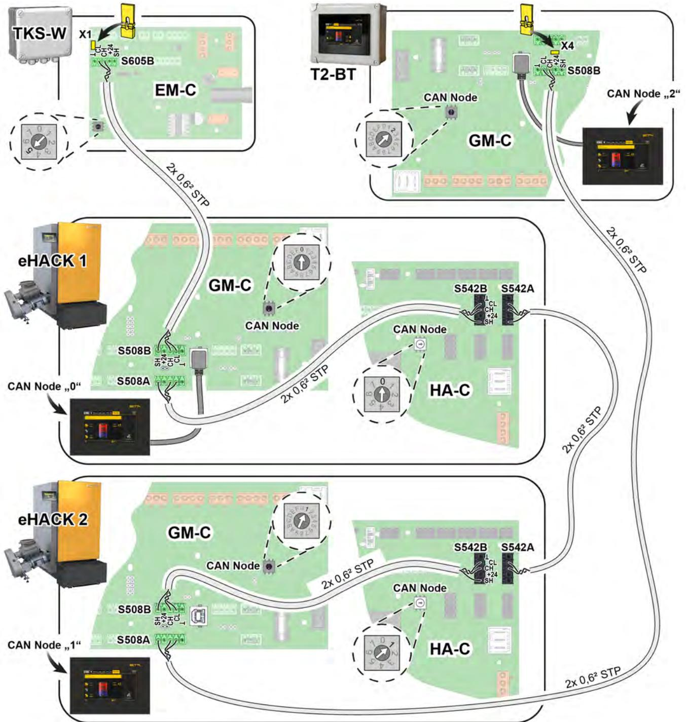
Fig. 5-1: CAN bus wiring
