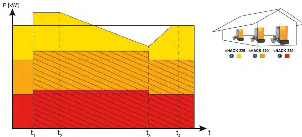
Fig. 4-1: De-ashing process with 3 boilers running
