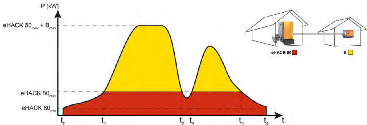
Fig. 4-3: Boiler with controllable burner
